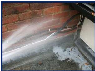
*Simulated rainfall testing of counter flashings*
